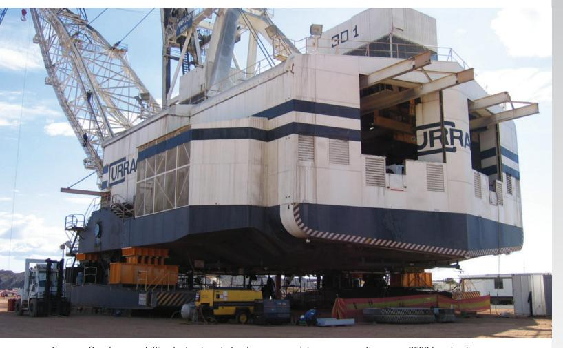
Enerpac Synchronous Lifting technology helped manage maintenance operations on a 3500 ton dragline crane in the Australian outback safely and efficiently. The automatic synchronous lifting operation separated the crane from its base so that slewing bearings could be replaced. Lowering and tilting cycles realigned bearing surfaces successfully, permitting the crane to be put back in operation quickly, reducing maintenance downtime.
