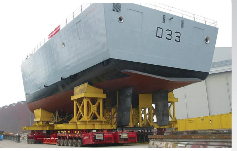
Hull sections for the UK Royal Navy's anti-air warfare destroyers are manufactured in 5 blocks, with the heaviest block weighing over 1400 ton. Prior to welding the blocks together to form the hull, the digitally controlled Enerpac Synchronous Lifting System lifts, weighs and positions the blocks, increasing efficiency and precision.
