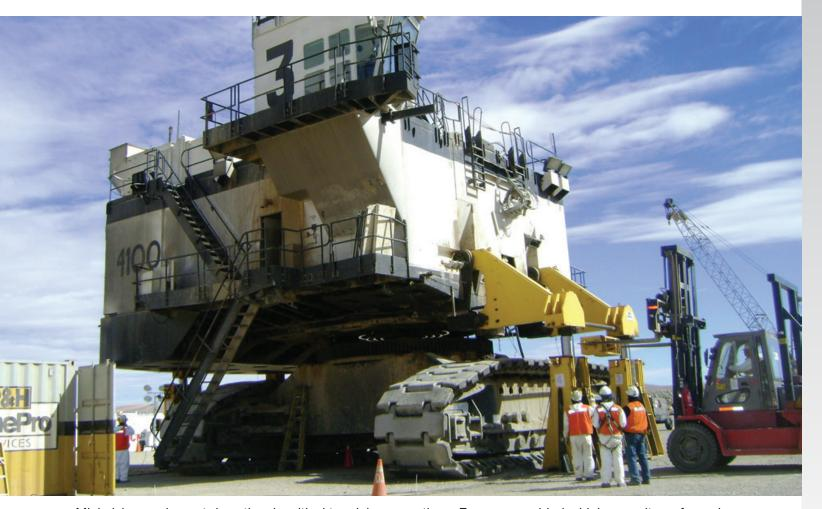
Minimising equipment downtime is critical to mining operations. Enerpac provided a high capacity, safe, and efficient shovel maintenance lifting method. The Enerpac Synchronous Lifting System automatically lifts and lowers cylinders in unison negating the need for multiple jack operators. Synchronous lifting has increased safety and productivity.
